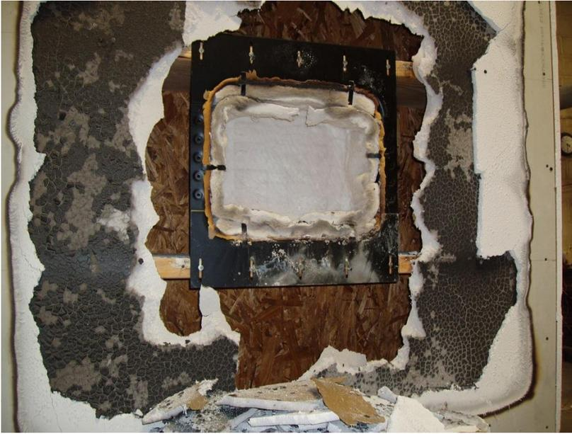
Joists & sub floor not charred after 1 hour test
