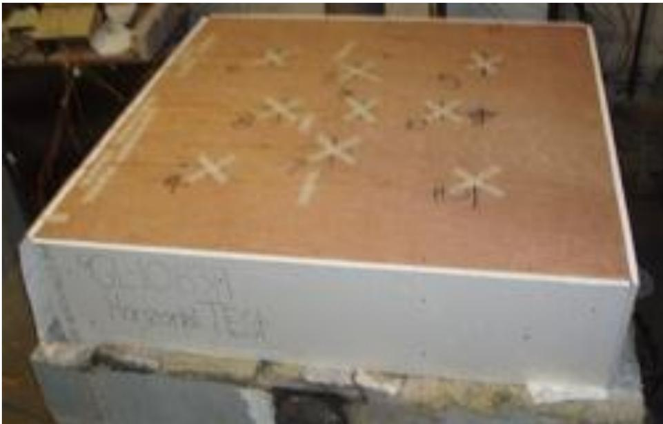
Unexposed surface after 1 hour test
