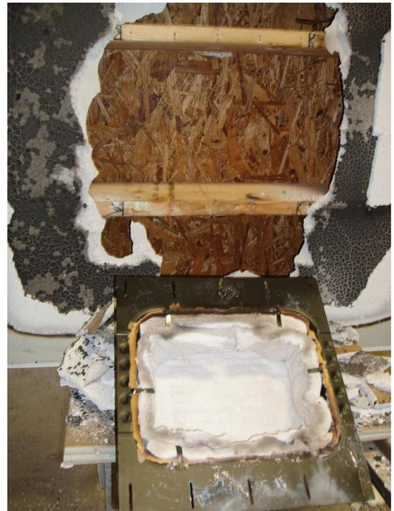
Back Box Removed—No char on floor assembly
