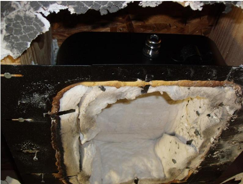
Grommet From Cable Hole Not Burned
